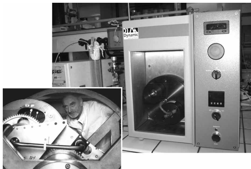
Figure 4. The smallest and the biggest hydrodynamic CCC columns available on the market (2007). Both columns are built by Dynamic Extraction, London, UK. The “Milli” is an 18 mL hydrodynamic column with one spool and a counterweight in a temperature regulated box. Lower left: The “Maxi” is a 5 liter double coil column. Ian Sutherland (Brunel University of West London) is shown inside the rotor to show the scale.
