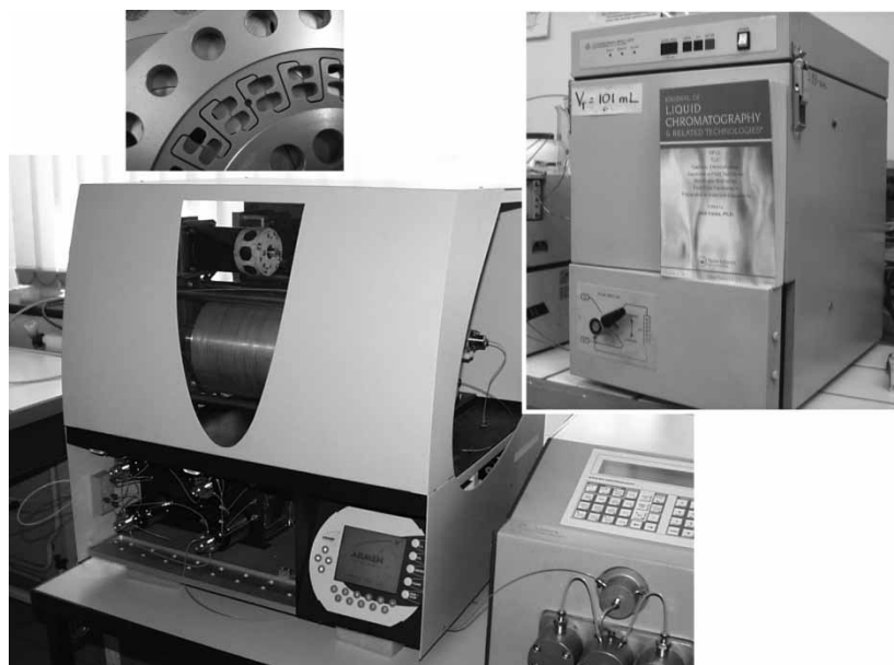
Figure 5. Hydrodynamic CCC column. Top right, the Sanki CPC-LLN, a 200 mL hydrostatic column sold for years in the US by Jack Cazes. The JLC&RT issue gives the scale. Bottom left: The Armen Elite one liter CPC (Armen Instruments, Vannes, France). Top left: close view of the patented dual chamber channel design of the Armen Elite CPC hydrostatic column.
